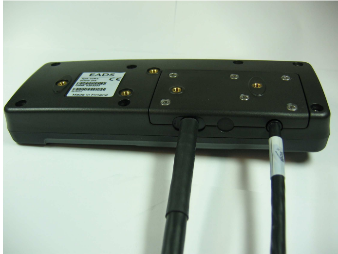
Figure 5 Fastened cable cover
